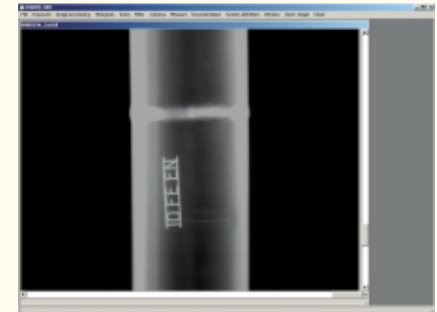
Fig. above: Welding with EN wire IQI
